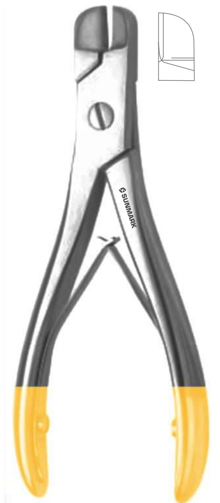
67-230-13 UltraCut™ TC Wire Cutting Plier For Soft Wires Up to Ø 1.5 mm For Hard Wires Up to Ø 1.0 mm Overall Length 13 cm (5 ¼")
