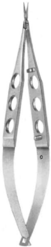
77-706-10 Gills-Vannas Micro Scissor Straight, Extra Thin Blades Sharp Tips 7 mm Long Blades With Max. 3 mm Cutting Edge Overall Length 10.5 cm (4")
